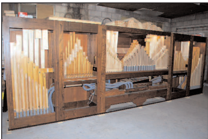
Figure 19. A contemporary Decap dance organ in progress, operated by a Palm Pilot and MIDI.
